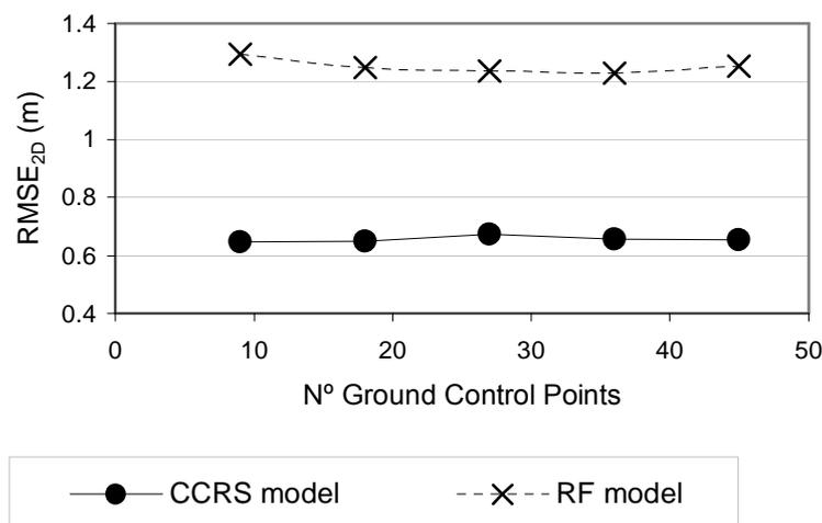
Figure 4: Planimetric Root Mean Square Error ( $RMSE_{2D}$ ) obtained in 79 ICPs by number GCPs using both 3D geometric correction models: Refined Rational Function (RF) and 3D multisensor physical geometric model developed at the Canada Centre for Remote Sensing (CCRS).
