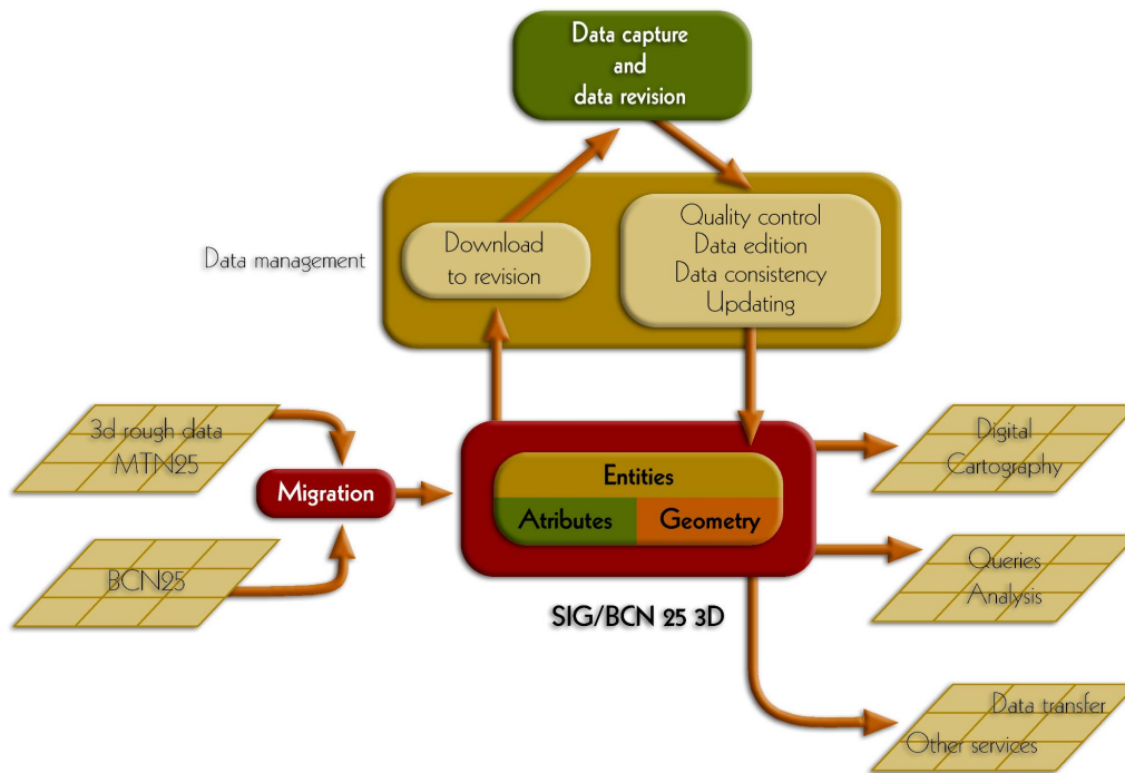
Figure 1: Integration of MAP (MTN25) and SIG (BCN25) data in an unified System.
