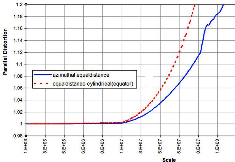
Figure 4, Scale-distortion graphs of Equidistant Projections
