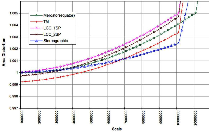
Figure 3, Scale- Distortion graphs in conformal projections
