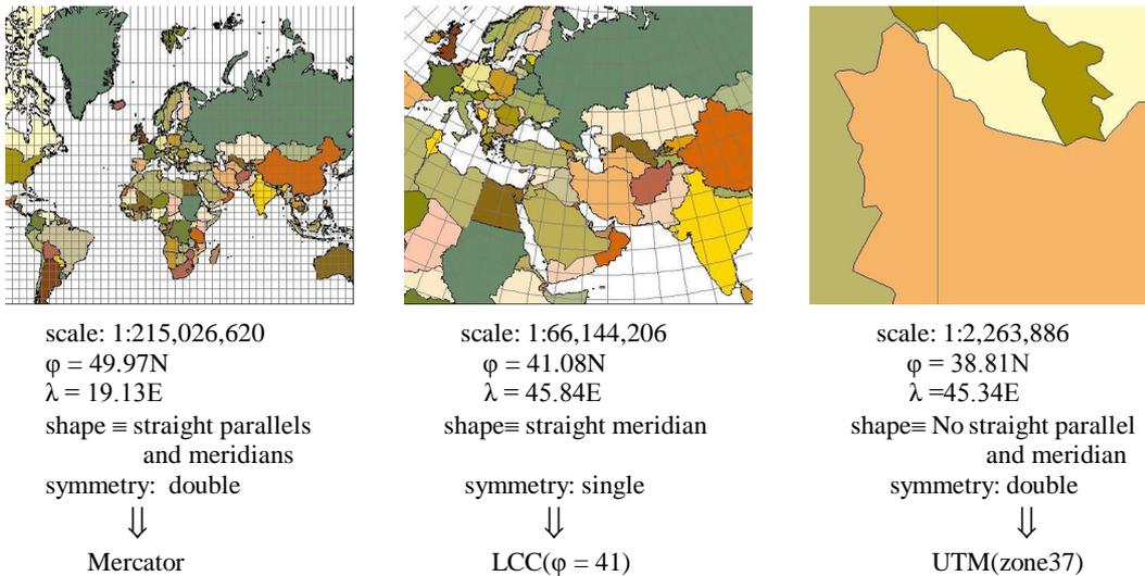
Figure 6, Samples of selecting the appropriate map projection in MMP
